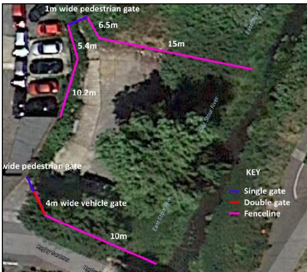
Figure 2 - aerial view showing fence/gate positioning
